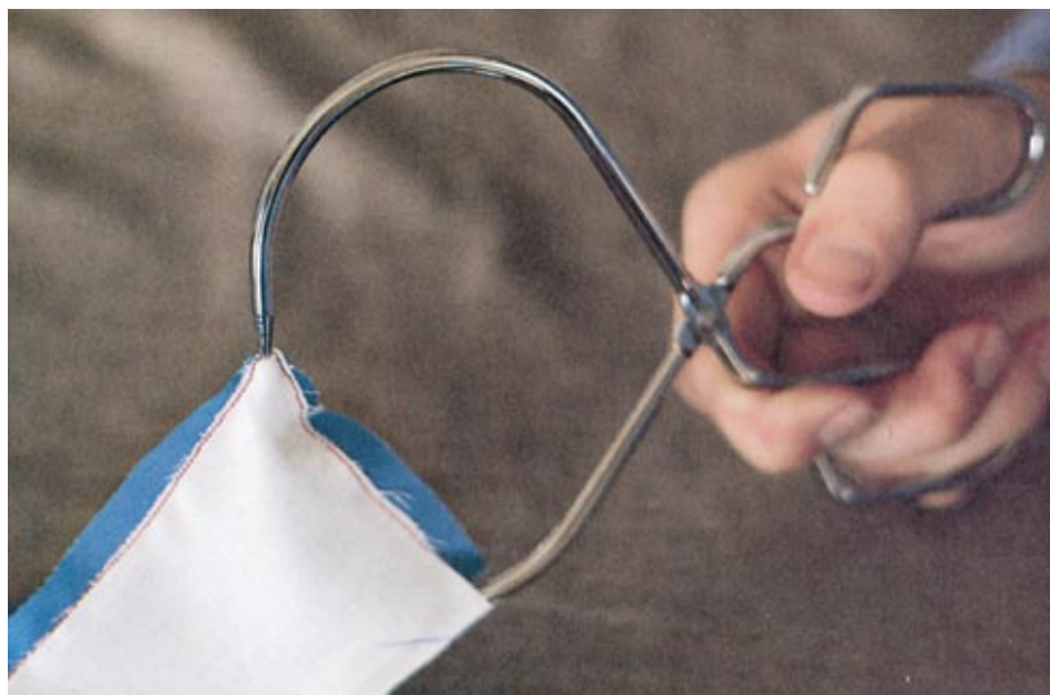
A point turner (above) pinches the fabric so that you can turn points without straining the fabric or poking through it. At right, Coffin wearing one of his shirts.
